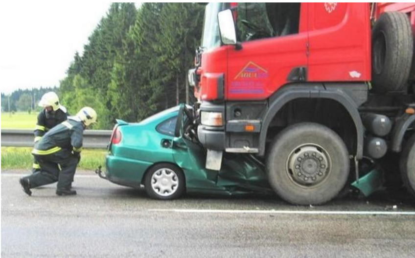
Example of collision with truck without under-run protection
