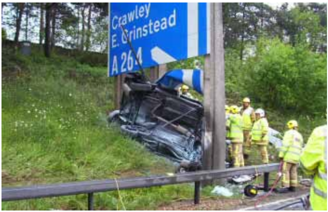
Figure 17: This photograph from the UK shows the unfortunate consequences of hitting a solid sign structure. Note the rigid crash barrier is also a hazard. Source: Passive Safety UK, http://www.ukroads.org/passivesafety
