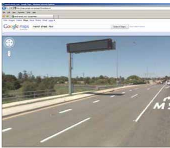
Figure 7: Example of a variable message sign on Marsh Street near Sydney's International Airport terminal. Electronic signs such as this should be proactively used to warn motorists of issues on the Eastern Distributor and the Harbour Bridge and Tunnel. Source: Google Maps, 2011.
