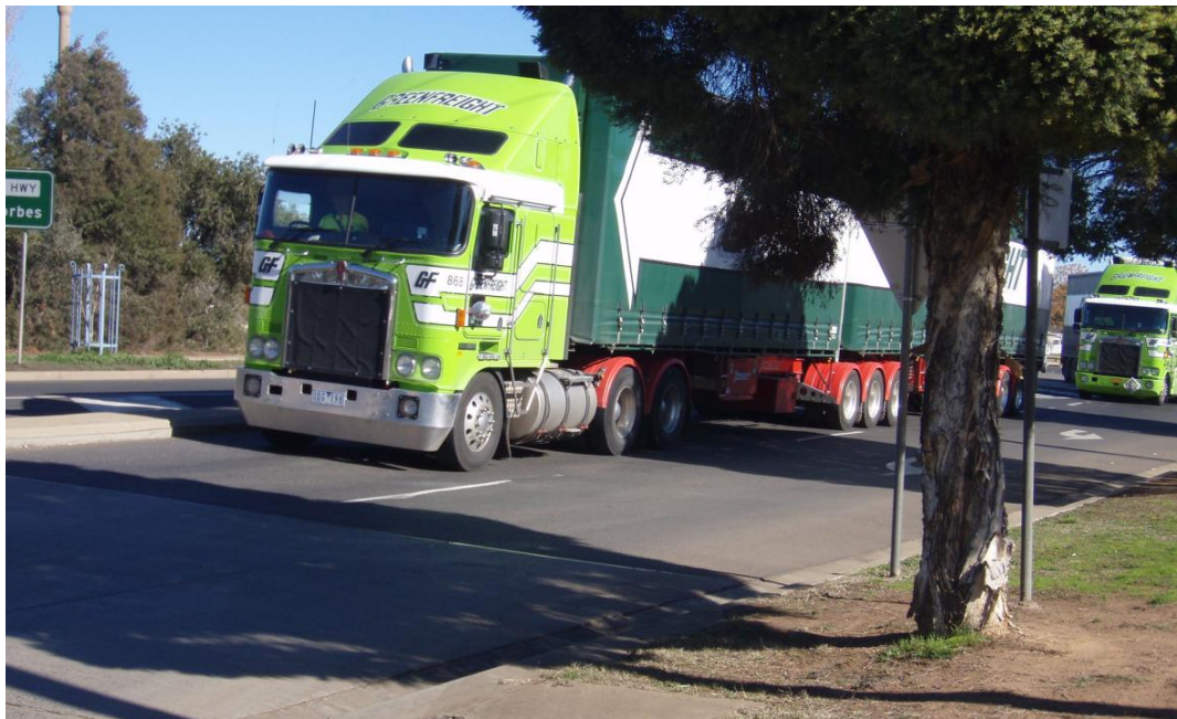
Figure 4-21 Two B-doubles approaching the hold line of the Hartigan Avenue/ Bogan Street intersection. Note the second vehicle is still within the control area of the Hartigan Avenue/ Forbes Street intersection.
