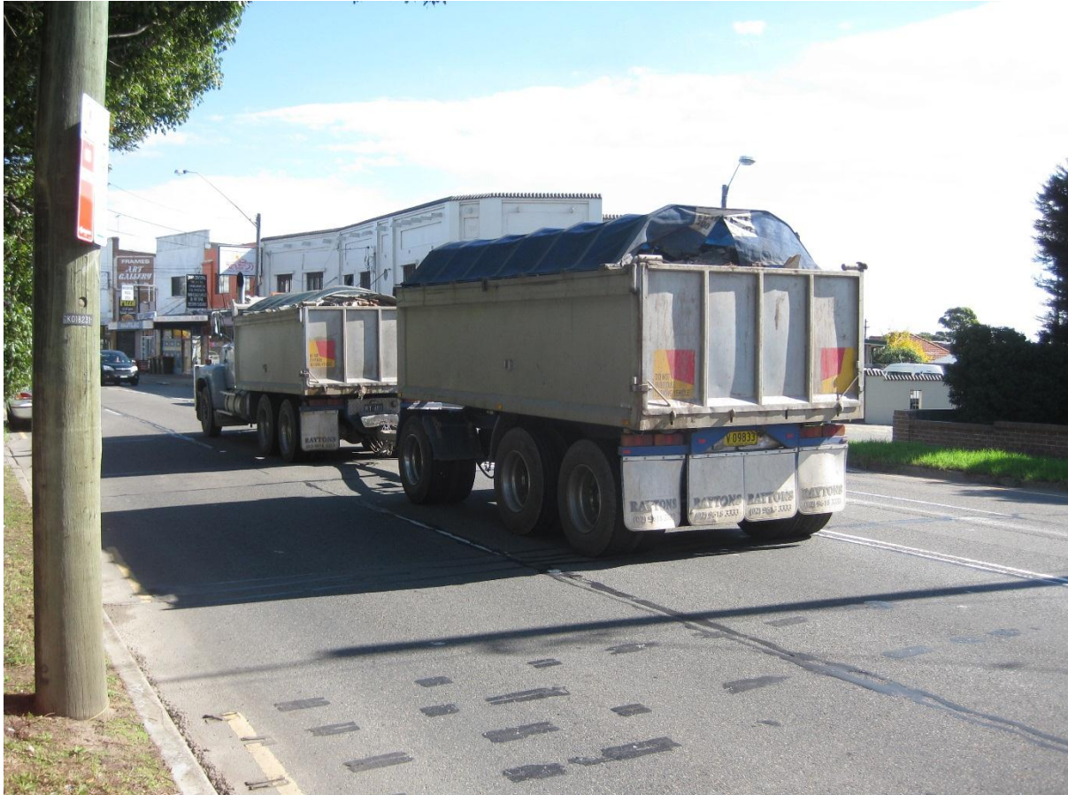
Photo of truck and dog trailer without retro-reflective strip or contour markings
